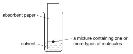
As the solvent rises up the paper, the molecules with the greatest solubility in the solvent travel a fixed distance up the paper. When the solvent reaches the top of the paper, the paper is removed, dried and sprayed with a dye. The different molecules appear as coloured spots.
